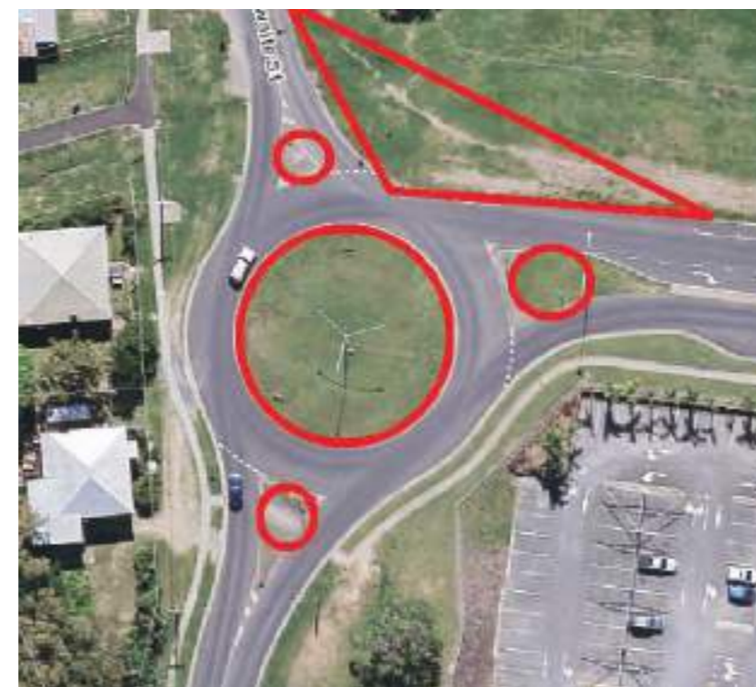
Figure 29. Priority 1. Junction of James Street and Braithwaite. The gateway statement needs to be installed in the roundabout and should be orientated to address north and south bound traffic. The other areas indicated in red require landscaping enhancement as a minimum intersection treatment. Broader enhancements are discussed in Section VII.F.2.
