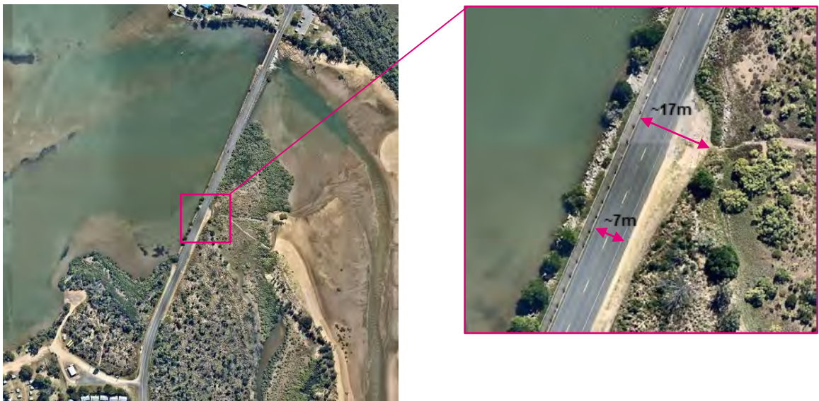
Figure 6-15 Restricted widths along causeway
