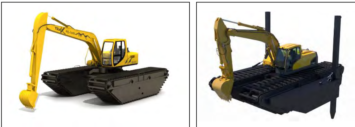
Figure 6-4 Amphibious excavator. Left : standard watertight pontoons, Right : supplementary pontoons with hydraulic-mechanical spud system
