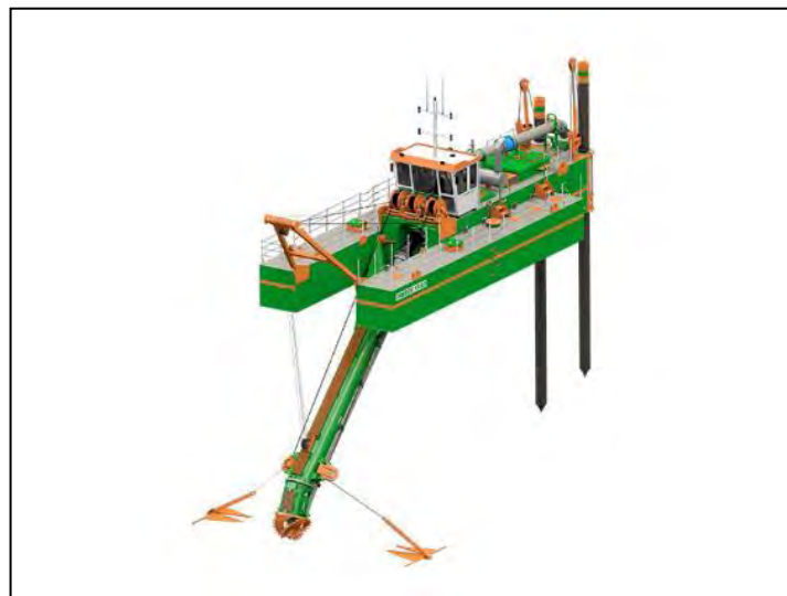
Figure 6-1 Typical cutter suction dredge configuration
