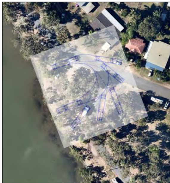
Figure 6-11 Schematic - Compatibility of the northern ramp area with a 19 m x 3.8 m trailer/truck combination
