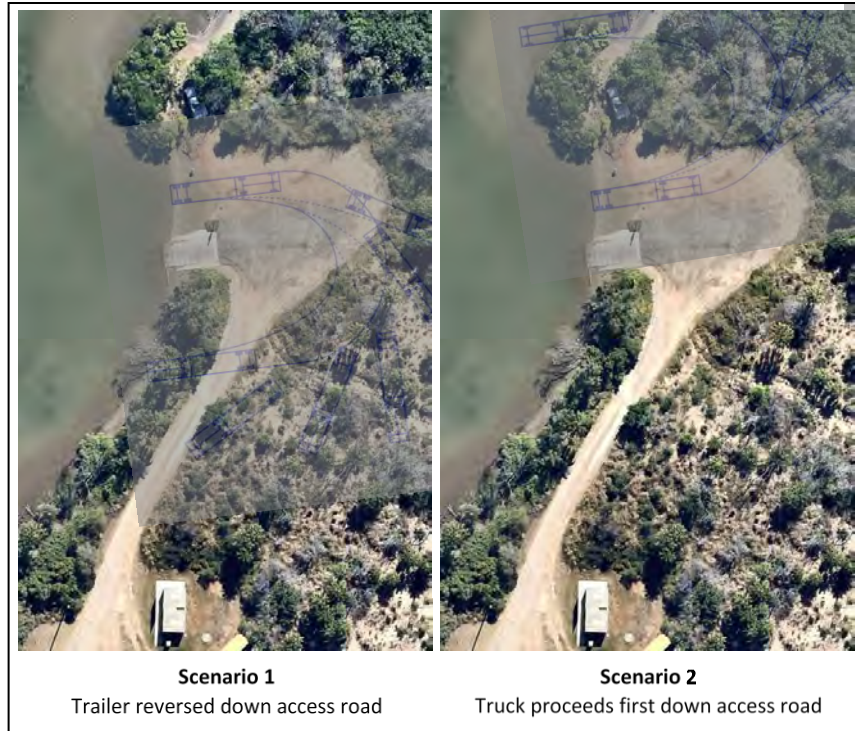
Figure 6-10 Schematic - Compatibility of natural ramp area with a 19 m x 3.8 m trailer/truck combination
