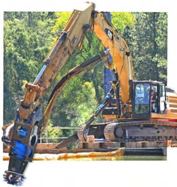
Figure 6-5 Amphibious excavator fitted with a rose cutter attachment (source: Eddy pump 2021)
